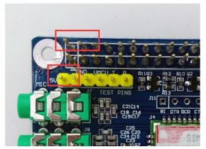
SIMCOM hardware manual for the module notes that it can draw up to 2A for short bursts. So get yourself a 5V 2A power supply and connect it via the DC socket.
