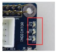
Nothing can happen until that magic three-second blink – so if that doesn't appear after a minute, something is wrong. Check your shield has the appropriate power supply, the antenna is connected correctly, and the SIM card is seated properly and locked in- and that your cellular account is in order. Finally, you may not have reception in that particular area, so check using a phone on the same network or move to a different location.
